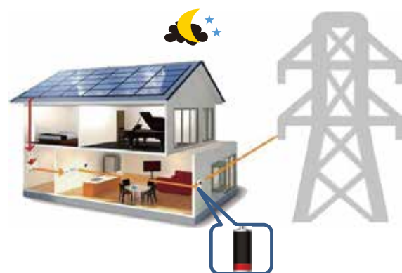
Late at night, the battery is off and the power grid supplies household appliances.
